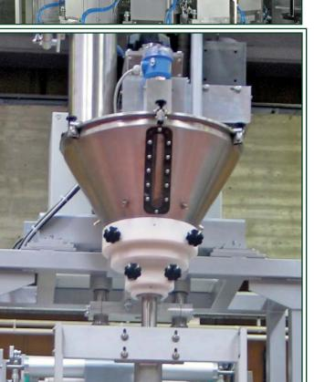
Filling of the bags with various systems according to the packed product (electonic scales with load cells or multihead scales, or auger fillers). Vibration of the finished bags.
