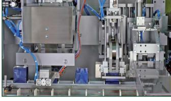
Bag top finishing on clearing conveyor. Finishing groups adjustment according to product density.
